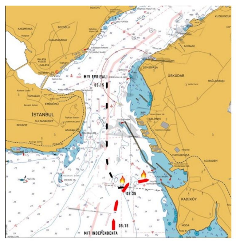
Figure 16. Estimated collision tracks and site of collision of M/V Evrivali and M/T Independenta
