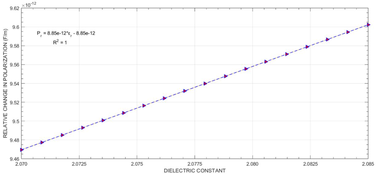
**Figure 4.** Relative change in polarization versus dielectric constant
