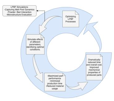
Figure 7. Digital twin application in laser powder bed fusion processes
