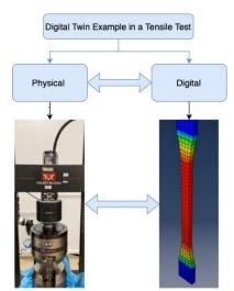
Figure 4. Digital twin application in a tensile test [34]
