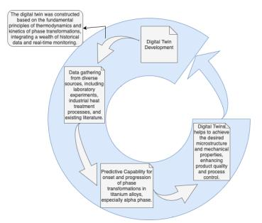
Figure 8. Digital Twin for predicting phase transformations in titanium alloys
