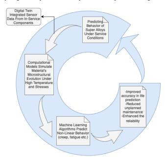
Figure 6. Application of digital twins in aerospace superalloys through material behavior prediction
