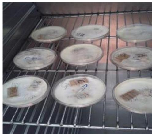
Figure 1. Fungal decay test
