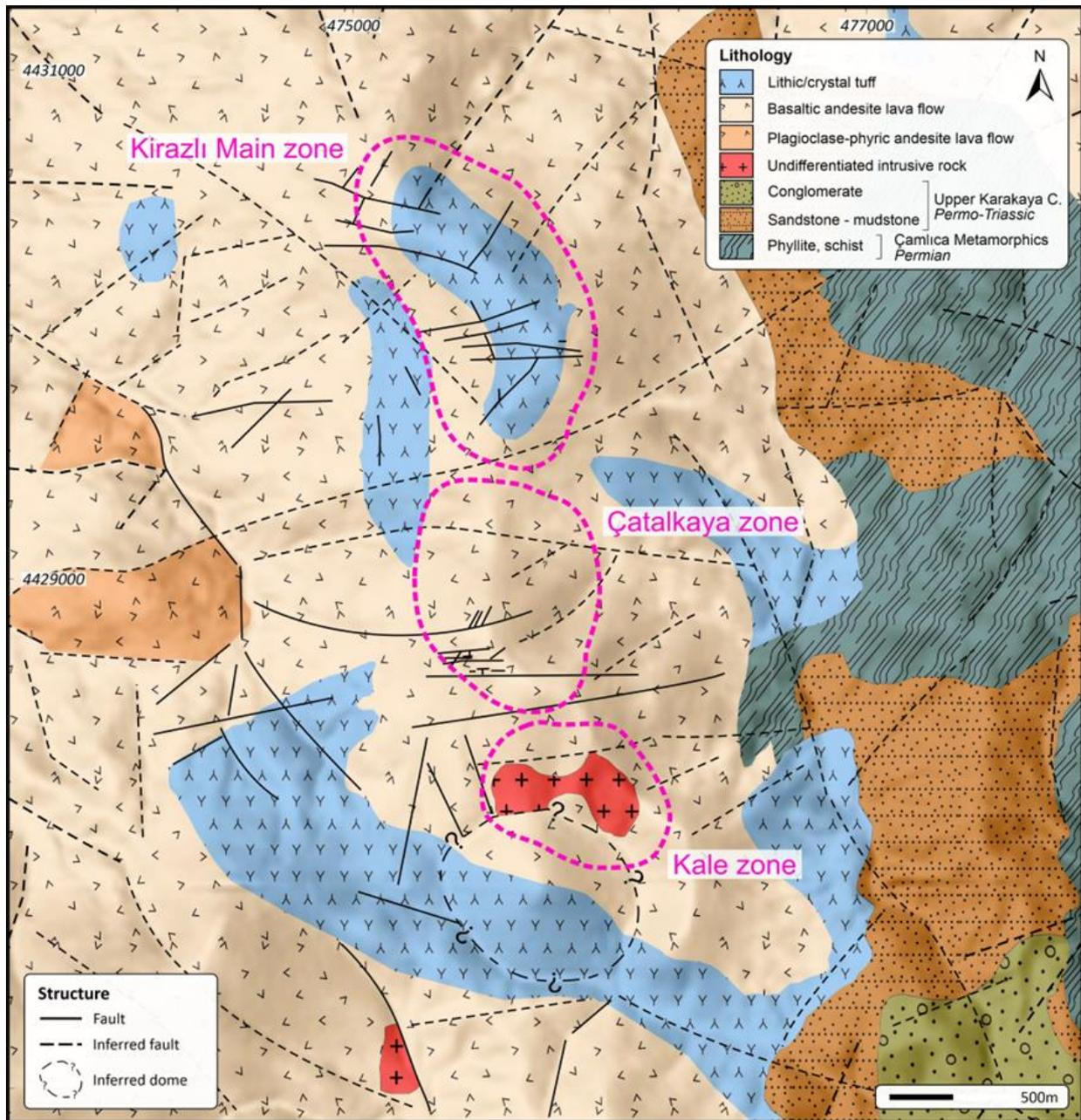
Figure 2. Geological map of the Kirazlı district showing lithological and structural elements
