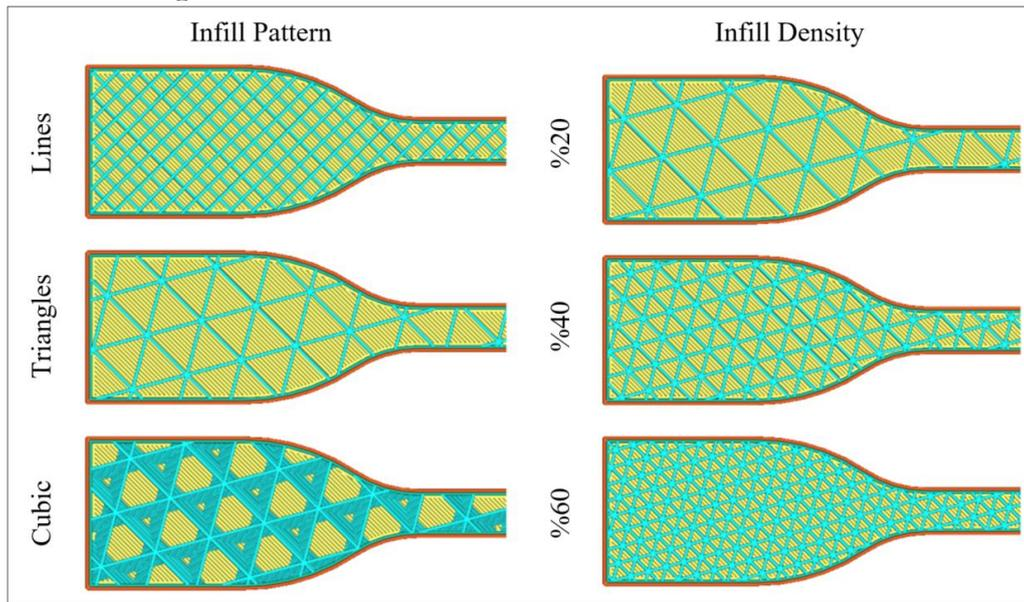
**Figure 1.** Infill pattern and infill density cross section views.
