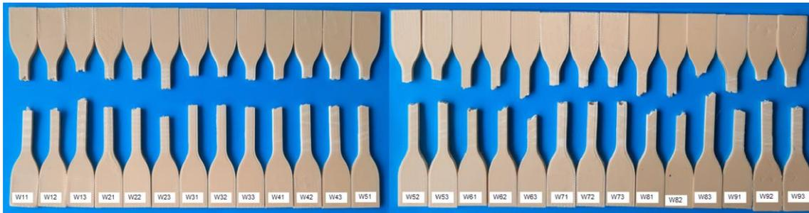
**Figure 3.** Image of tensile test specimens after testing.
