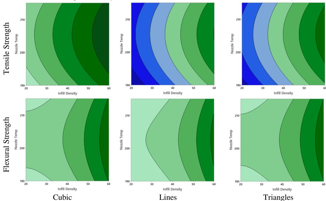
**Figure 6.** Contour Plot graphs of the relationship between printing parameters and mechanical strength criteria.
