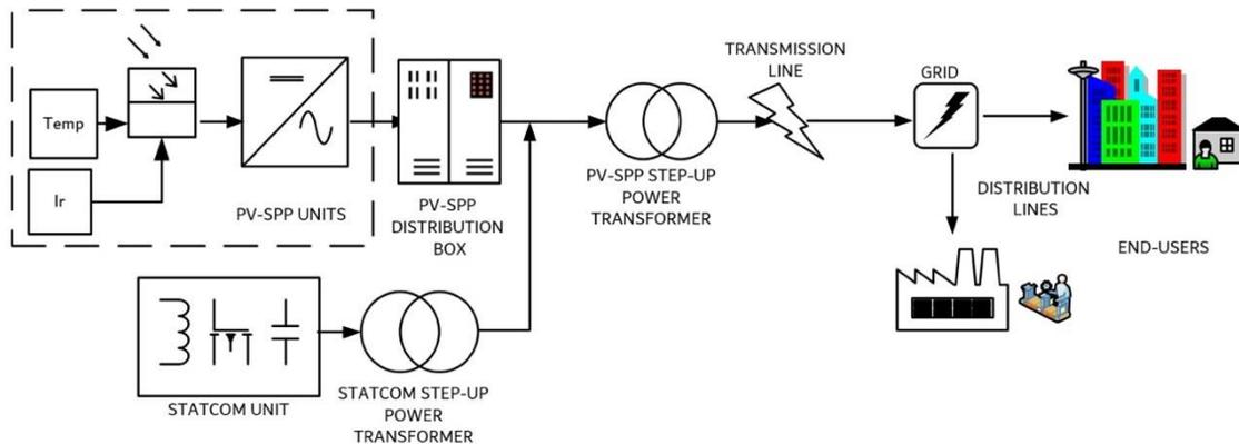
Figure 4. Single-line diagram of optimised PV-SPP
