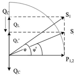
Figure 5. AC Powers vector diagram pre & post RPC
