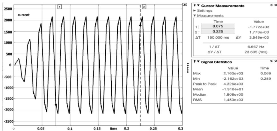
Figure 12. Post-STATCOM system current waveform
