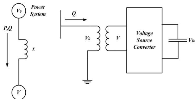
Figure 6. Operating Principle of the STATCOM.
