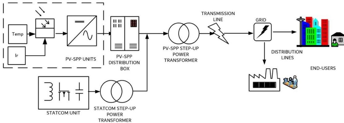
Figure 4. Single-line diagram of optimised PV-SPP
