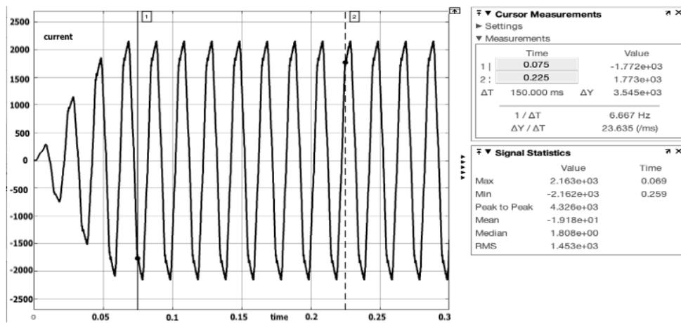
Figure 12. Post-STATCOM system current waveform
