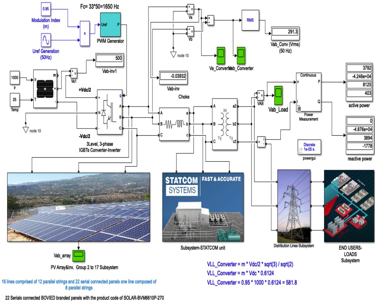
Figure 3. MATLAB-Simulink modelling of the optimised system
