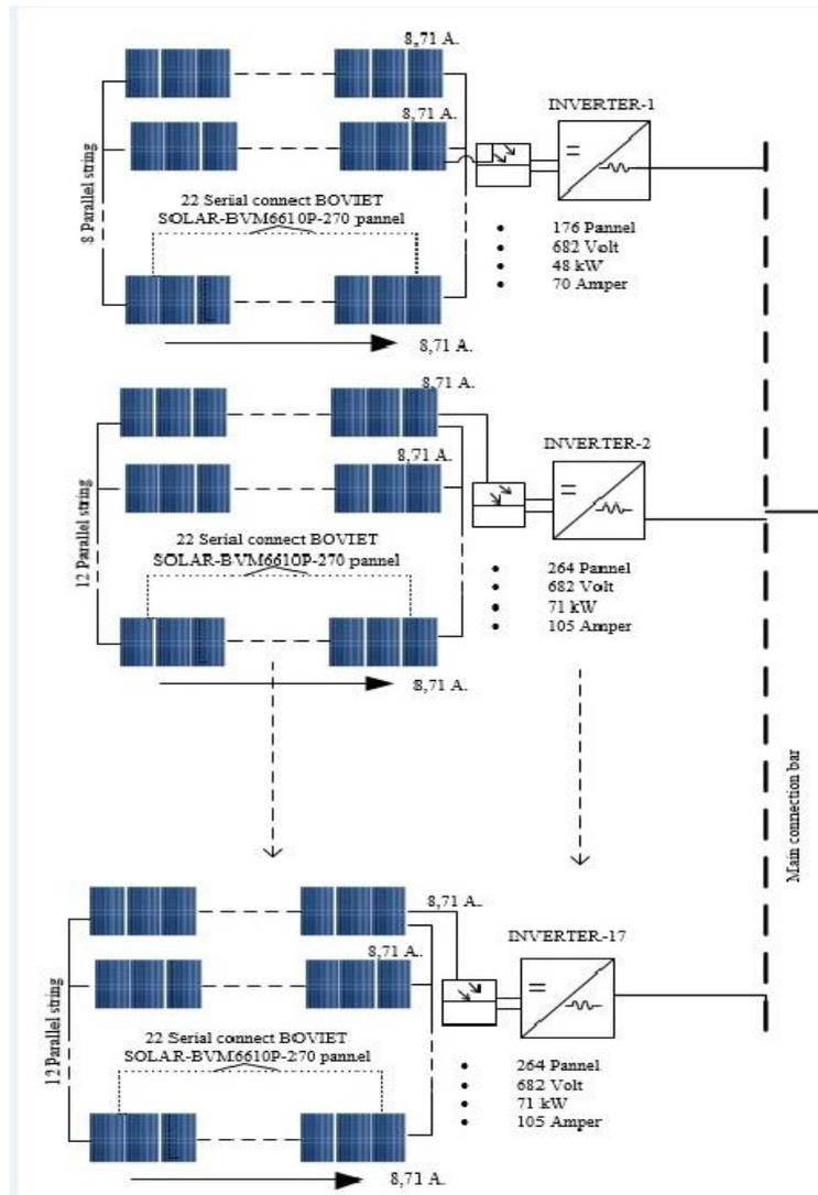
Figure 2. Single-line diagram of PV Strings
