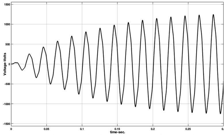
Figure 10. After STATCOM system voltage waveform
