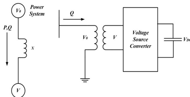
Figure 6. Operating Principle of the STATCOM.
