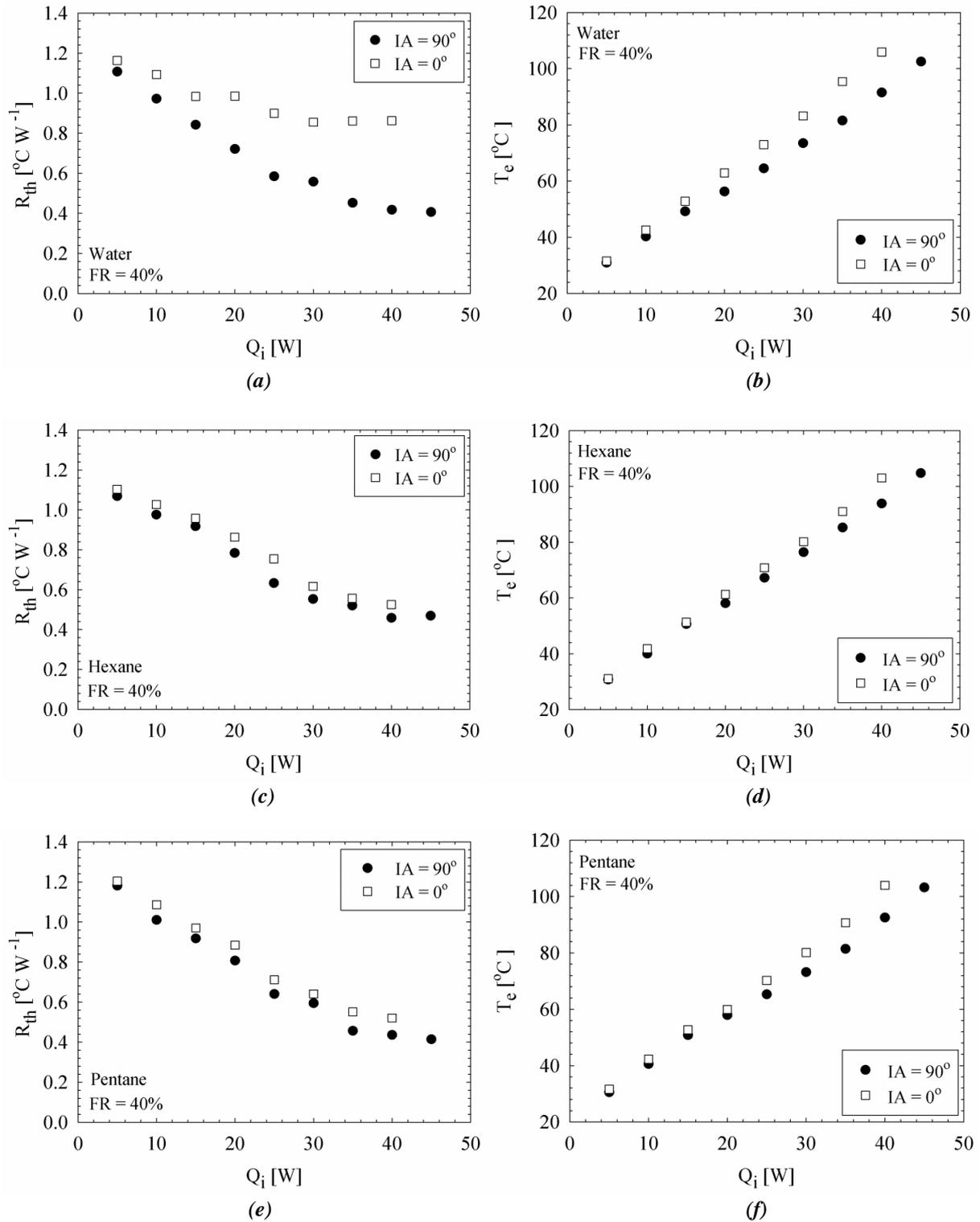
**Figure 6.** Influence of gravity on performance of the FP-CLPHPs charged with pure fluids.
