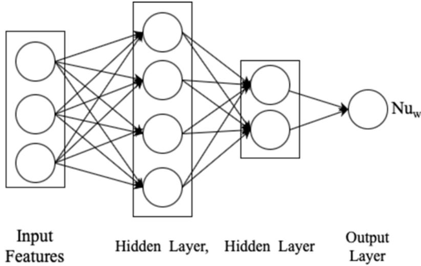
**Figure 5.** Structure of the proposed Multilayer Perceptron.
