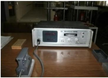
Fig 5. Thermal conductivity meter unit
