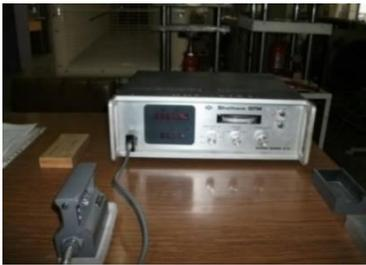
Fig 5. Thermal conductivity meter unit
