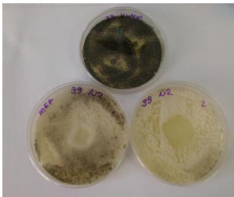
**Figure 1.** The petri dishes of control (up) and UT-1 (uniaxial electrospun thyme oil, 1 cm x1 cm) (on the left) and UT-2 (uniaxial electrospun thyme oil, 2 cm x 2 cm) (on the right) against 39-04X4
