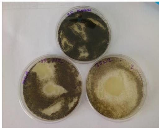
**Figure 4.** The petri dishes of control (up) and UT-1-X1 (uniaxial electrospun thyme oil, 1 cm x 1 cm) (on the left) and UT-2-X1 (uniaxial electrospun thyme oil, 2 cm x 2 cm) (on the right) against 35-03X1
