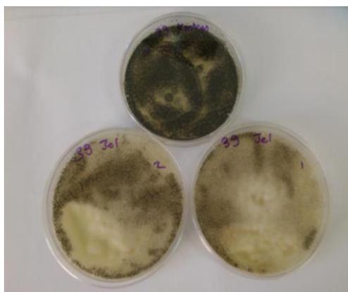
**Figure 3.** The petri dishes of control (up) and uniaxial electrospun gelatin with 2 cm x2 cm (on the left) and uniaxial electrospun gelatin with 1 cm x 1 cm (on the right) against 39-04X4
