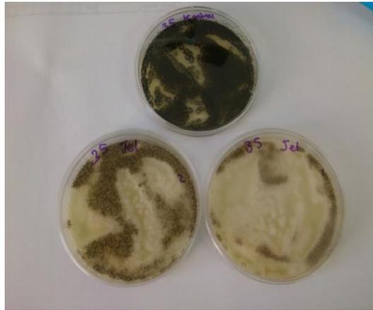
**Figure 6.** The petri dishes of control (up) and uniaxial electrospun gelatin with 2 cm x2 cm (on the left) and uniaxial electrospun gelatin with 1 cm x 1 cm (on the right) against 35-03X1
