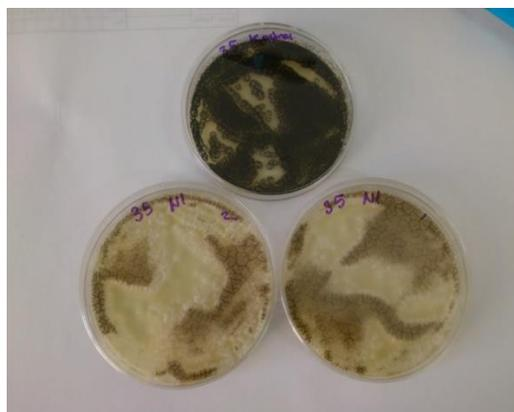
**Figure 5.** The petri dishes of control (up) and CT-1-X1 (coaxial electrospun thyme oil, 1 cm x 1 cm) (on the left) and CT-2-X2 (coaxial electrospun thyme oil, 2 cm x 2 cm) (on the right) against 35-03X1
