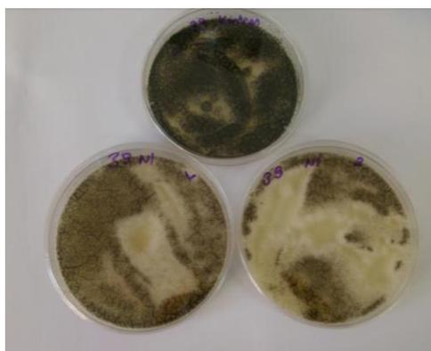
**Figure 2.** The petri dishes of control (up) and CT-1 (coaxial electrospun thyme oil, 1 cm x1 cm) (on the left) and CT-2 (coaxial electrospun thyme oil, 2 cm x 2 cm) (on the right) against 39-04X4.
