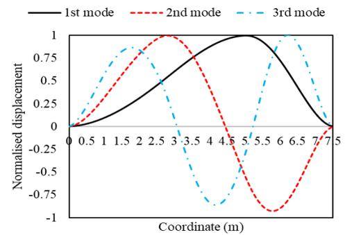
**Figure 6.** First three mode shapes of segmented Timoshenko beam on Pasternak foundation with F-F boundary conditions ( $K_W = 50, K_S = 4$ )
