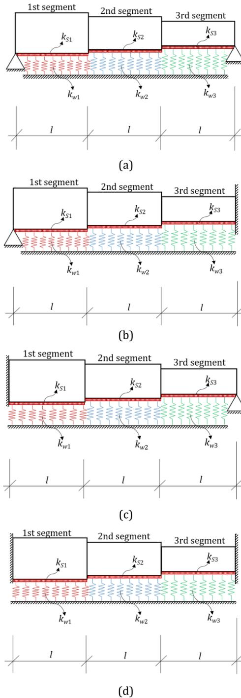
Figure 2. Mathematical model of segmented Timoshenko beam on Pasternak foundation for a) S-S b) S-F c) F-S d) F-F boundary conditions
