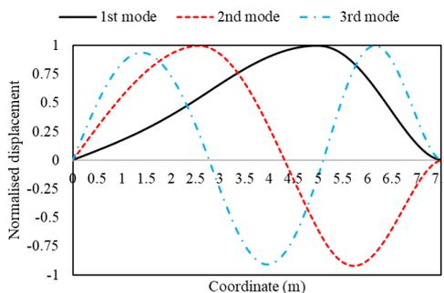
**Figure 4.** First three mode shapes of segmented Timoshenko beam on Pasternak foundation with S-F boundary conditions ( $K_W = 50, K_S = 4$ )
