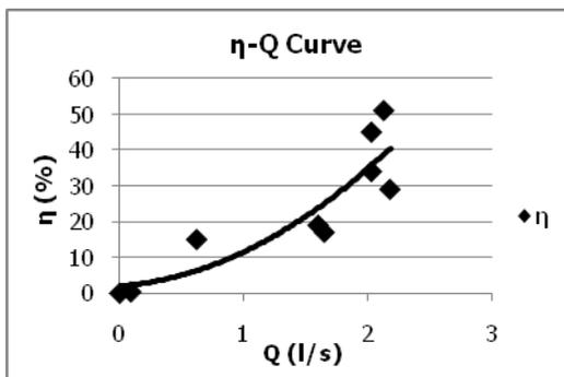
Figure 4. Manometrical efficiency-debit curve measured before the experiment
