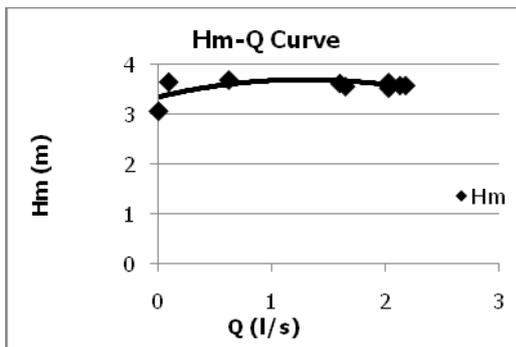
Figure 2. Manometrical height-debit curve measured before the experiment
