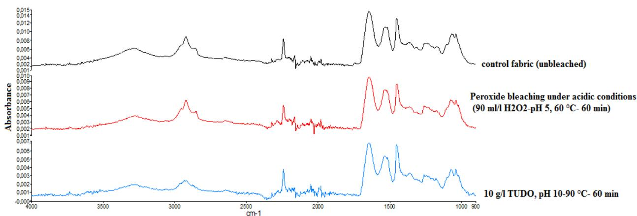
Figure 12. FTIR-ATR Analysis of milk casein fabric samples
