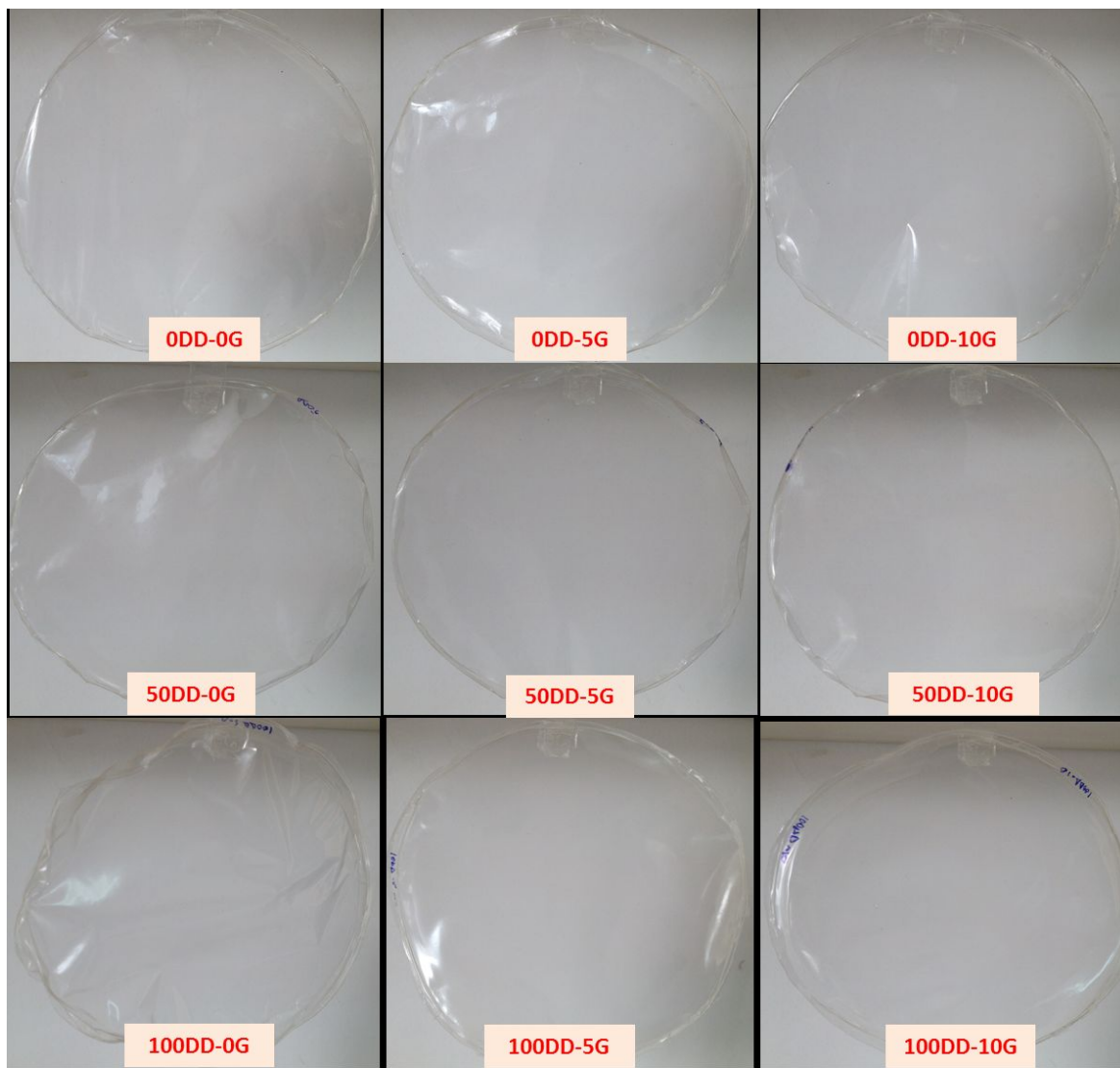
Figure 2. Physical appearance of salep glucomannan film samples as a function of deacetylation degree (DD, %) and glycerol content (G, %)
