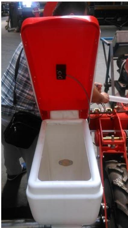
**Figure 7.** The montage of ultrasonic distance meter on seed tank
