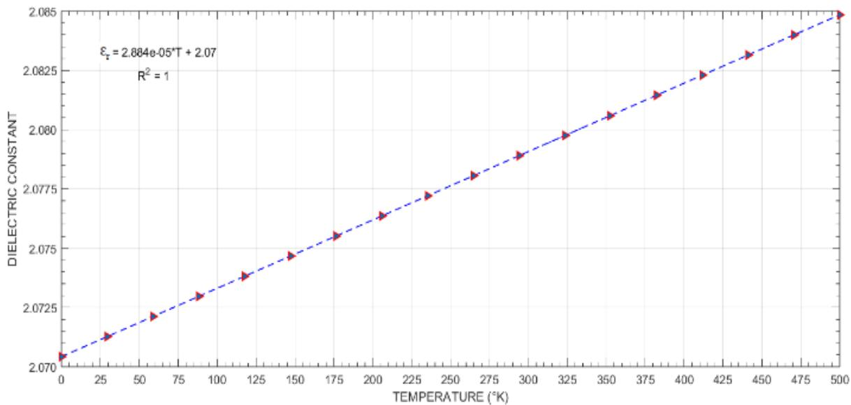
**Figure 2.** Dielectric constant versus temperature
