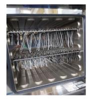
*Figure 6. Placing and Suspension of the EPR test pieces inside the ageing oven.*
