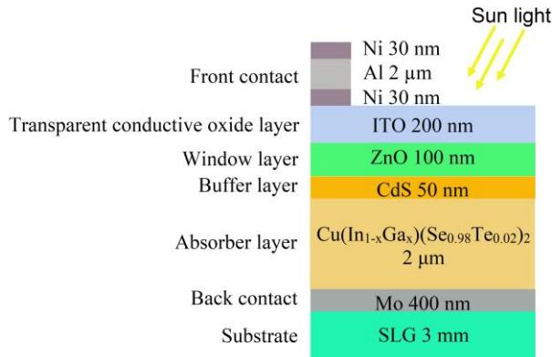
Figure A: Schematic illustration of the thin film solar cell / Şekil A: İnce film güneş pilinin sematik gösterimi
