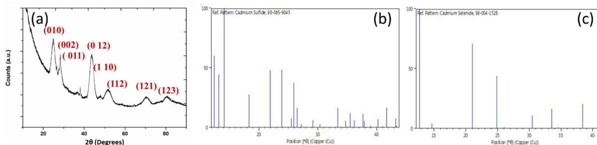
**Figure 3.** XRD pattern of synthesized NRs (a), reference peak positions of CdS (b), reference peak positions of CdSe (c).
