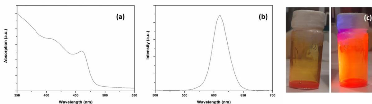
**Figure 2.** Absorption (a) and photoluminescent (b) spectra of NRs. Digital images of synthesized NRs under daylight (left) and UV-light excitation (right) (c).
