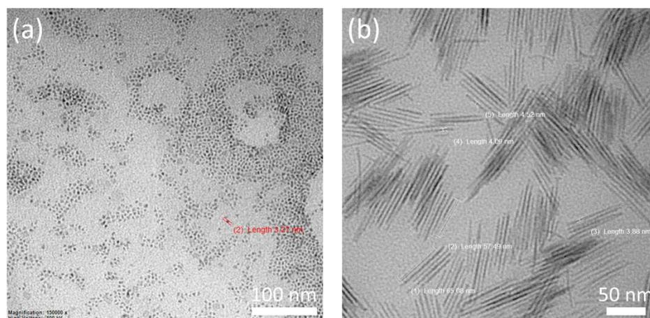
**Figure 1.** TEM images of CdSe quantum dots (a), and NRs (b).
