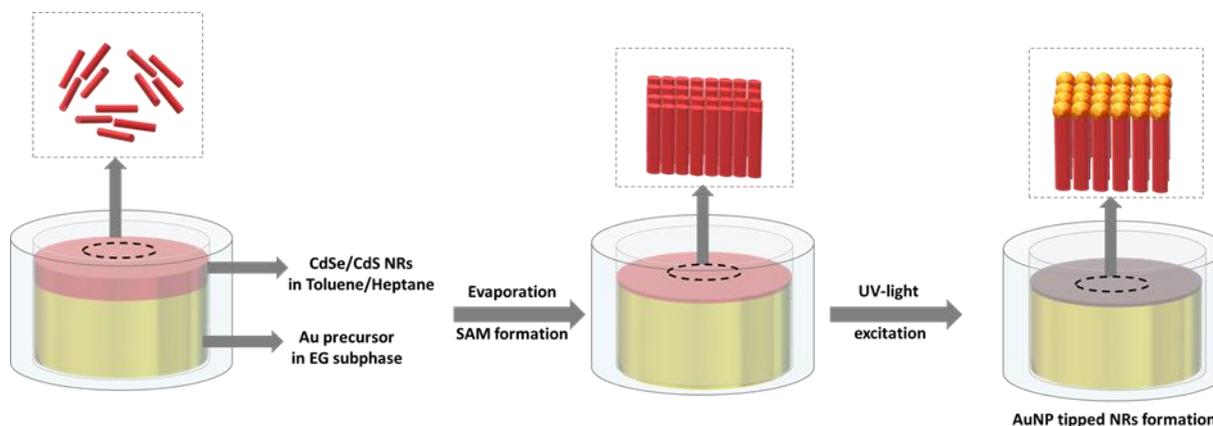
**Figure 4.** Preparation steps of Au-tipped CdSe/CdS NRs on the subphase
