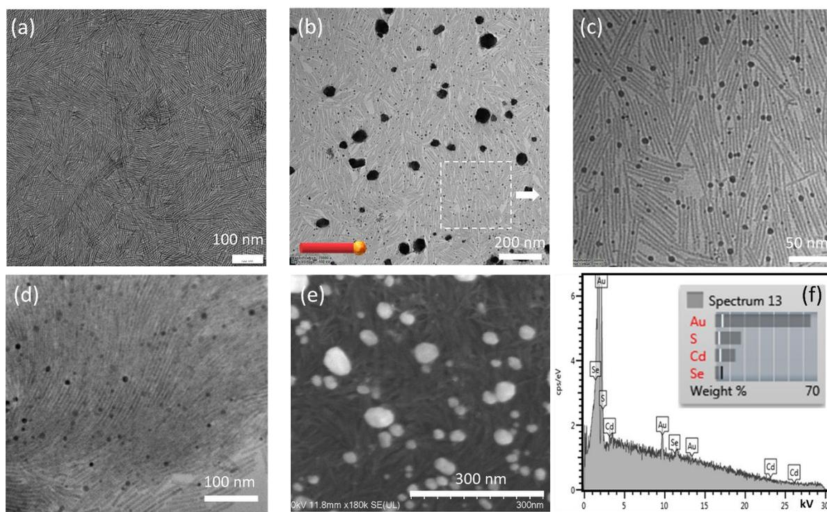
**Figure 5.** TEM images of self-assembled NRs (a), gold-tipped NRs (b,c) and smaller gold tipped NRs (d). SEM image of gold tipped NRs (e) and EDS analysis of the gold-tipped NRs film on silicon wafer (f).
