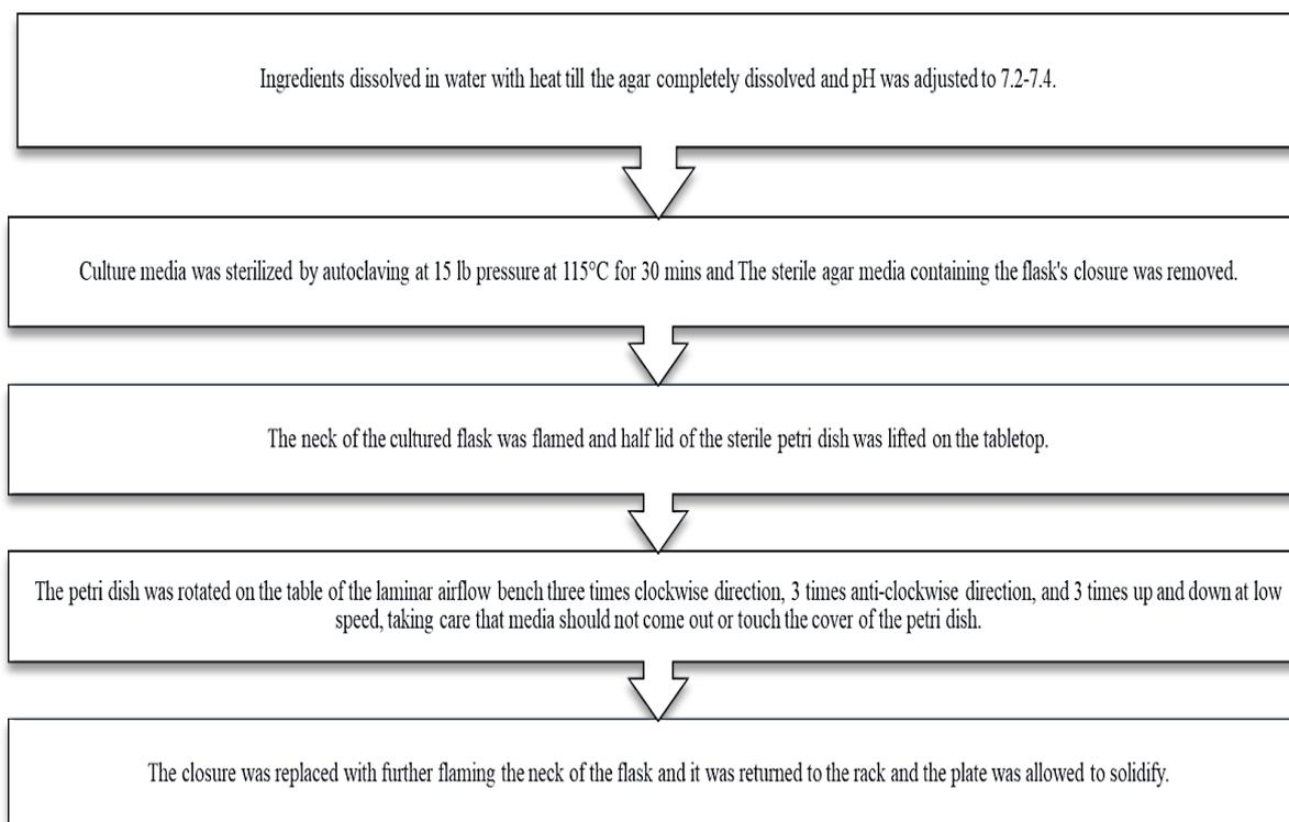
Figure 2. Sterilized agar plate preparation for microbial assay.
