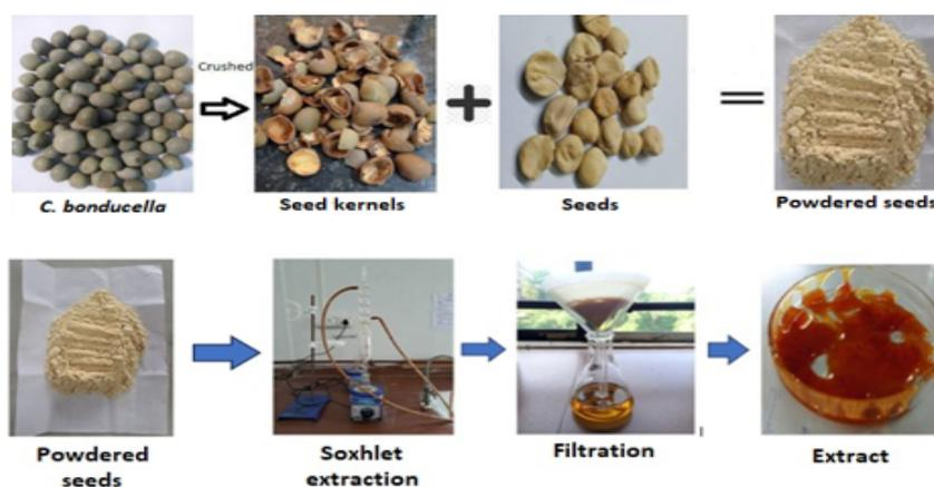
Figure 1. Extraction of *Caesalpinia bonducella* through Soxhlet apparatus.
