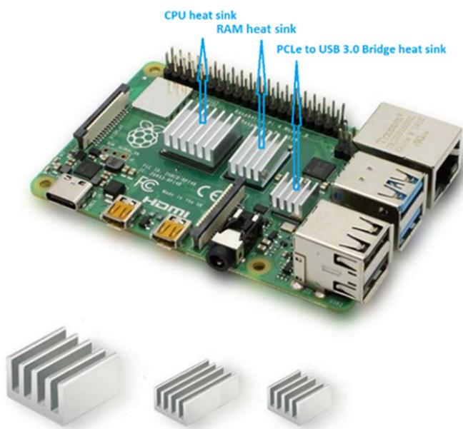
**Figure 1.** Raspberry Pi with heat sink usage points
