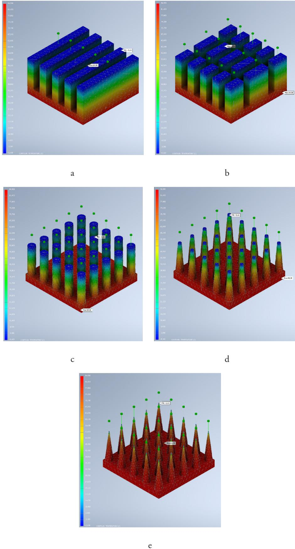
Figure 8. Thermal analysis results of five different PCLe to USB 3.0 Bridge heat sink models with aluminum material
