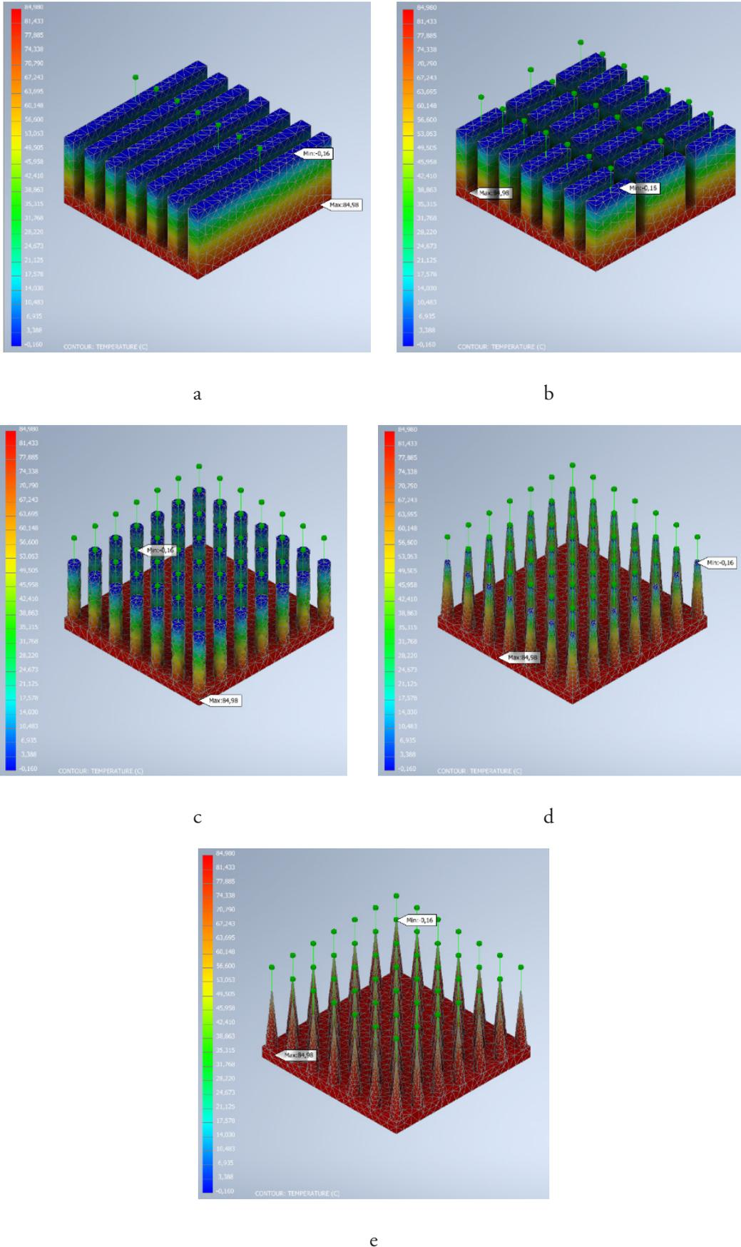
Figure 4. Thermal analysis results of five different CPU heat sink models with aluminum material
