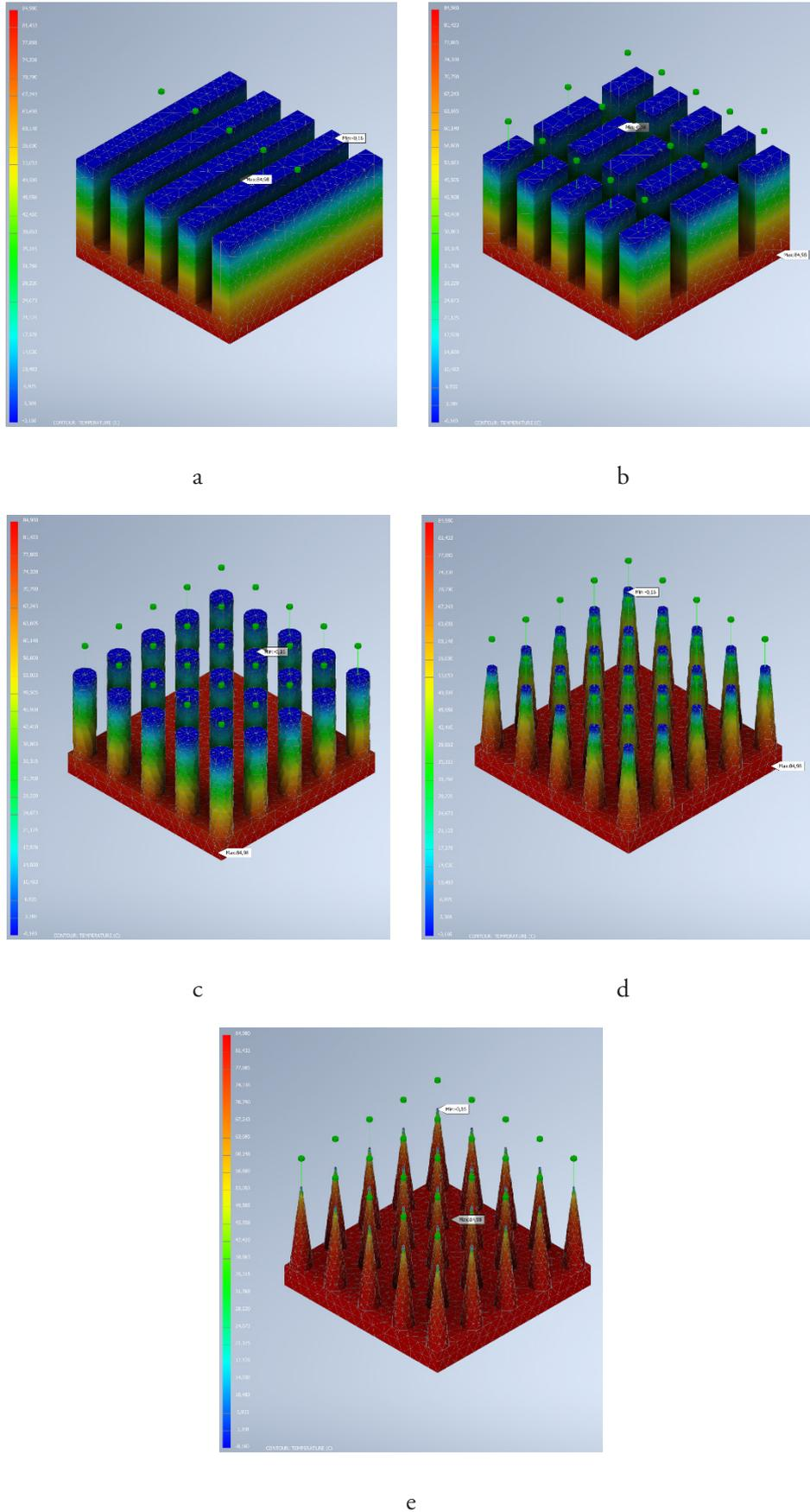
**Figure 9.** Thermal analysis results of five different PCLe to USB 3.0 Bridge heat sink models with copper material
