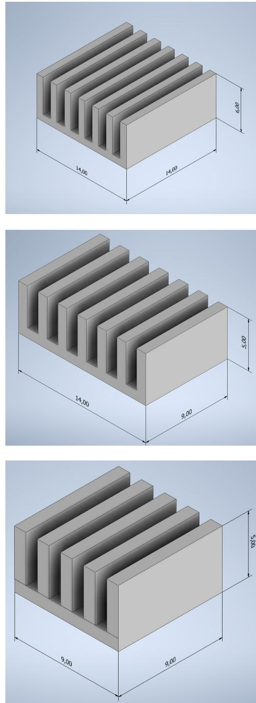
**Figure 2.** Dimensions of the designed heat sink models
