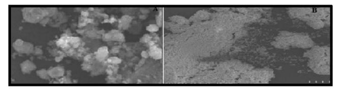
Figure 1. Scanning electron microscopy (SEM) micrographs of A) MWCNT, B) ZrO<sub>2</sub> NPs
