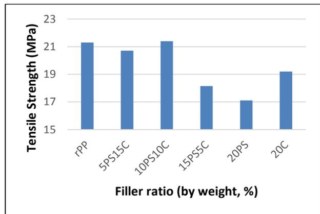
**Figure 2.** Tensile strength properties of composites materials
