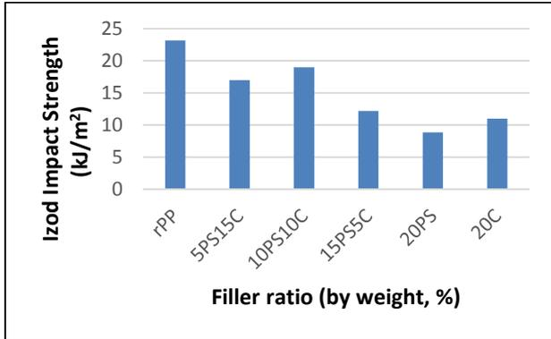
Figure 3. Izod impact strength properties composite samples
