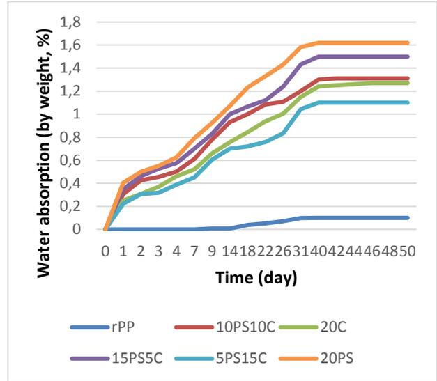
Figure 5. Water absorption properties of composites samples
