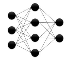
Input layer Hidden layer Output layer **Figure 2.** Example of Single Layer ANN Layers (Kızrak, 2018)
