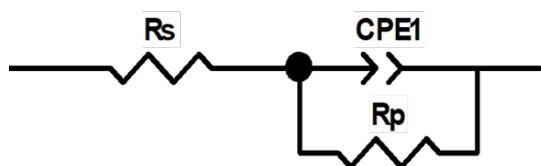
**Figure 5:** Equivalent Circuit for brass without inhibitor and with presence of inhibitor FTSC.
