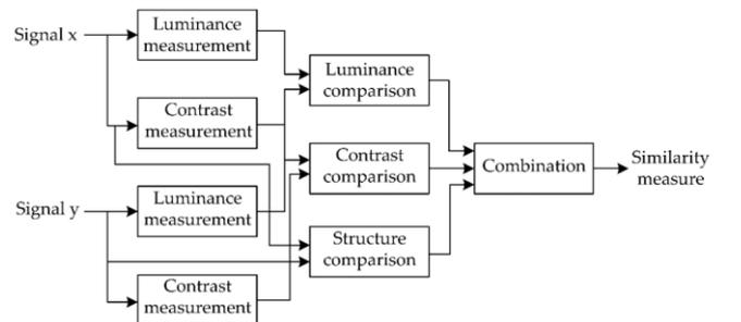
Figure 5. Schema of SSIM
