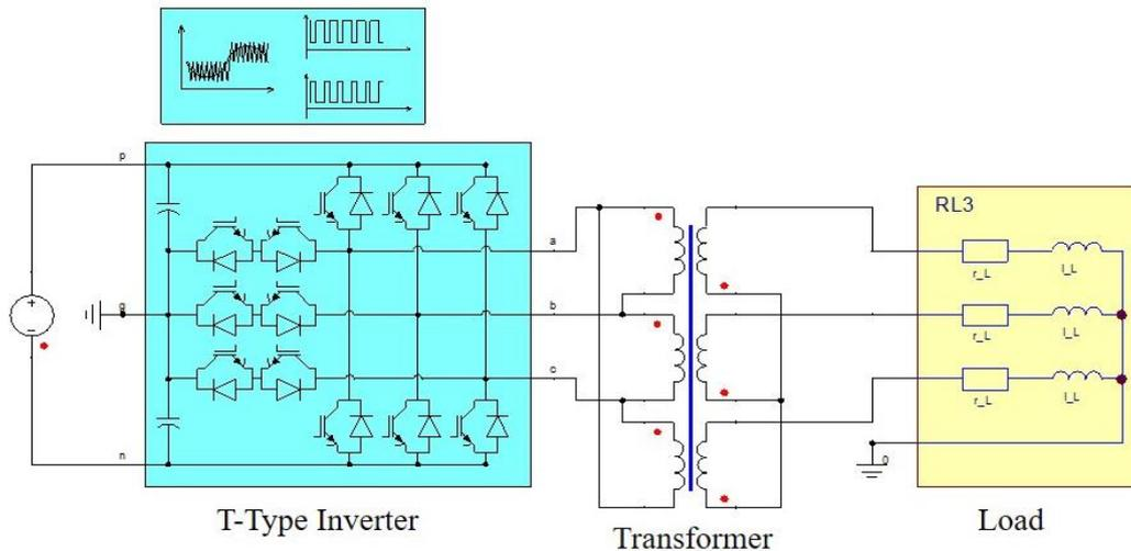
Figure 1. The circuit topology of the transformer with a T-type inverter.
