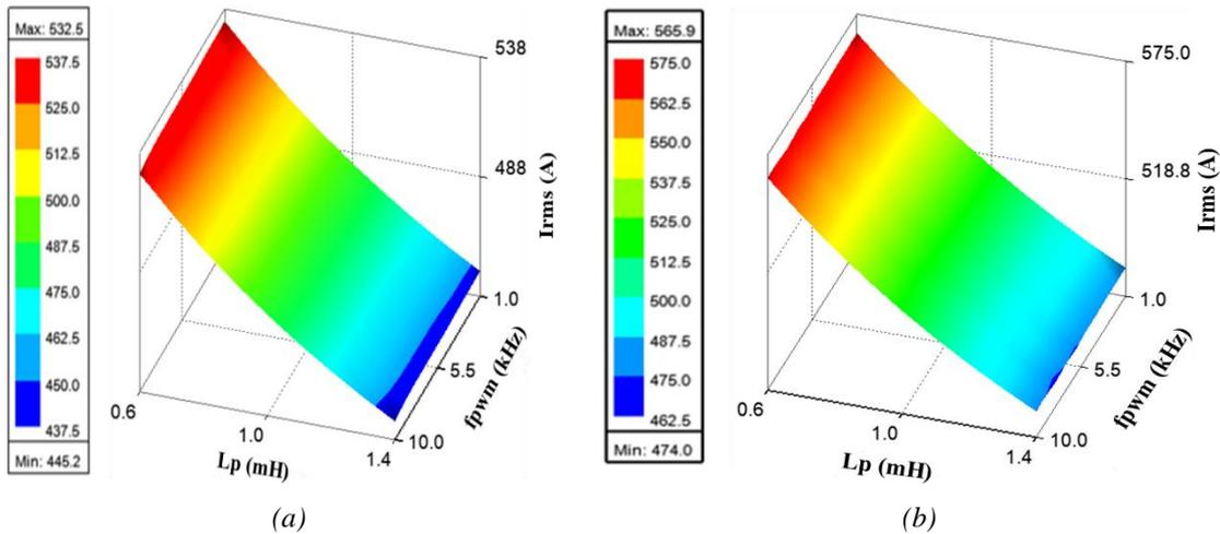
Figure 8. Output currents on the surface of PWM frequency and  $L_p$ : a)  $m_r=0.8$  and b)  $m_r=0.85$ .
