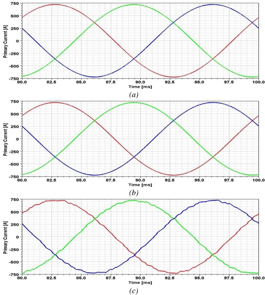
Figure 6. Primary current  $m_r=0.85$ ,  $t_{dead}=0.1 \mu s$  of a)  $f_{pwm}=10 \text{ kHz}$ , b)  $f_{pwm}=5 \text{ kHz}$ , c)  $f_{pwm}=1 \text{ kHz}$ .
