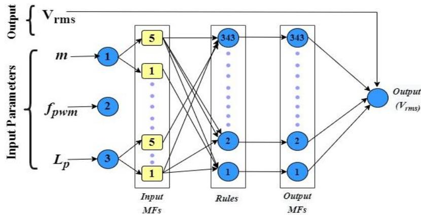
Figure 2. The ANFIS Model Structure
