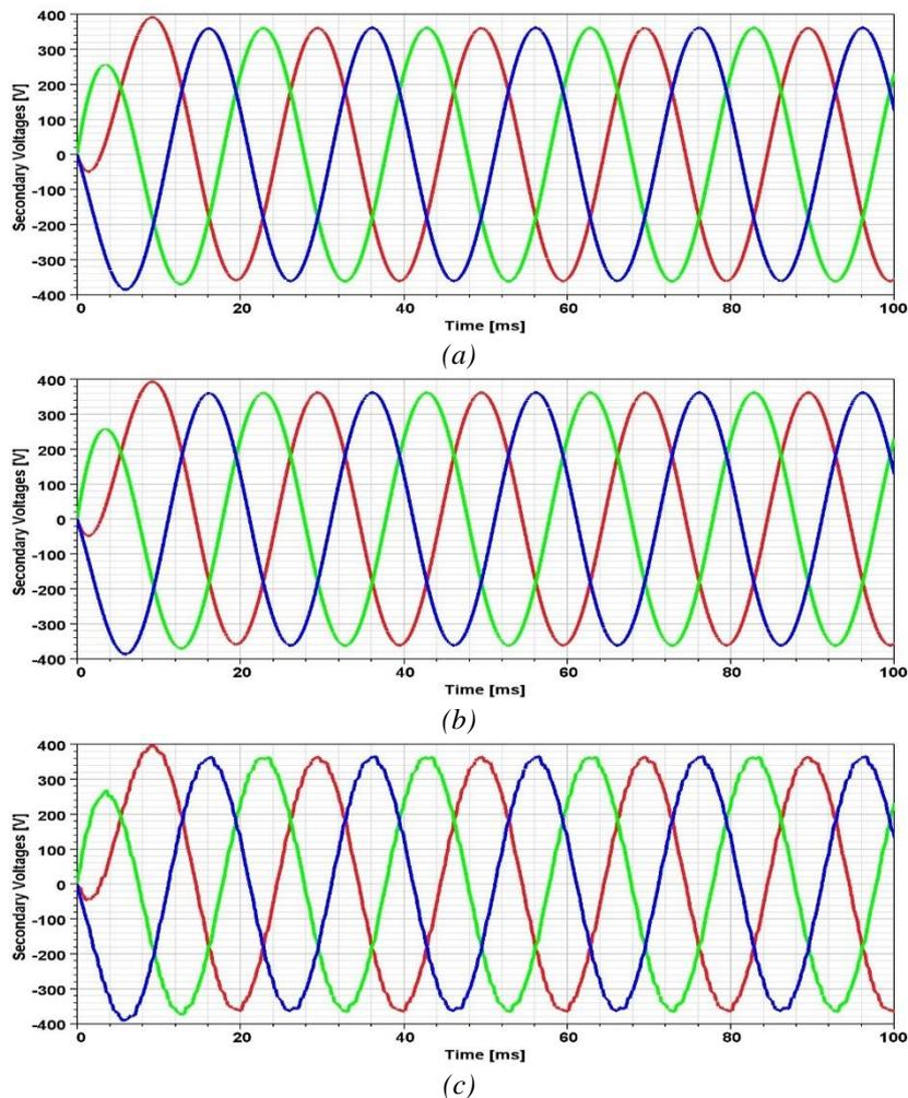
Figure 5. Secondary voltages  $m_r=0.85$ ,  $t_{dead}=0.1 \mu s$  of a)  $f_{pwm}=5 \text{ kHz}$ , b)  $f_{pwm}=10 \text{ kHz}$ , c)  $f_{pwm}=1 \text{ kHz}$ .
