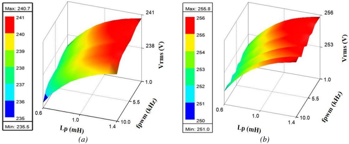
Figure 7. Output voltages on the surface of PWM frequency and  $L_p$ : a)  $m_r=0.8$  b)  $m_r=0.85$ .
