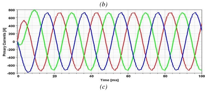
Figure 4. Primary currents  $m_r=0.85$ ,  $t_{dead}=0.1 \mu s$  of a)  $f_{pwm}=5 \text{ kHz}$ , b)  $f_{pwm}=10 \text{ kHz}$ , c)  $f_{pwm}=1 \text{ kHz}$ .
