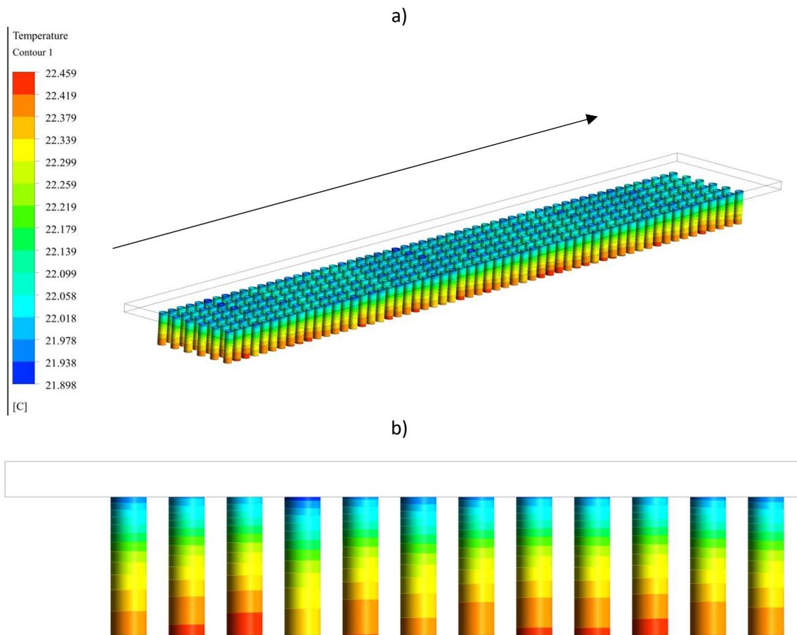
**Figure 4.** Cold Plate Cooling Method Temperature Distribution a) General View b) Detail View
