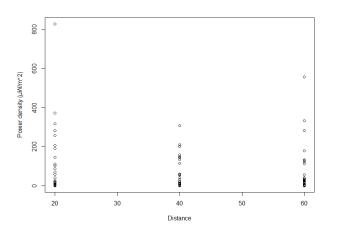
Figure 5. Base station power density distribution according to distances.
