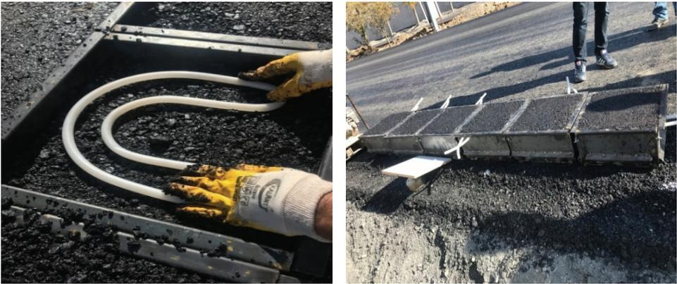
*Figure 1 - Preparation of asphalt samples with hydronic heating system*
