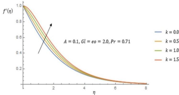
**Figure 5.** Influence of porosity constraint,  $k$  on the fluid flow rate
