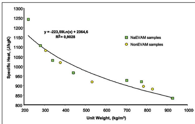
Figure 8. Density versus Cp value of tested samples.
