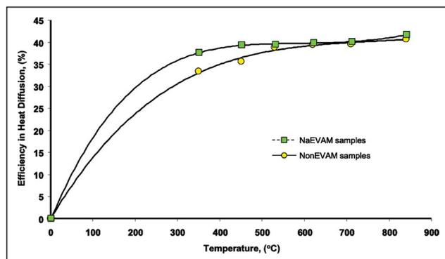
**Figure 10.** Heat dissipation efficiency against heating temperature.
