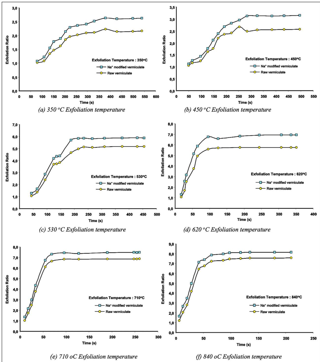
**Figure 1.** Influence of heating time on exfoliation ratio at different temperatures.
