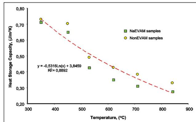
Figure 9. Heating temperature and heat storage capability relationship.
