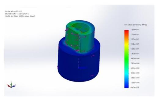
Figure 5. Stress graph of the generated key model.
