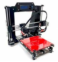
Figure 2. RepRap Prusa 3D printer [8].
