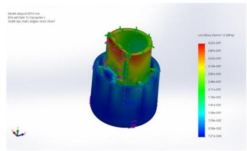
Figure 4. Stress graph of the broken key model.
