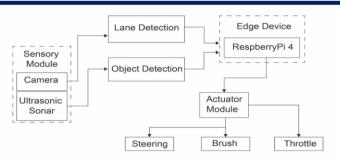
Fig. 1. The agent architecture of self-driving road cleaner
