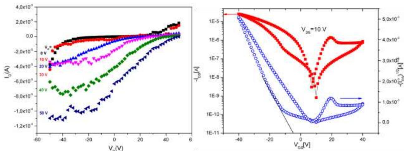
Figure 2. a) Output characteristic and b) Transfer characteristic of OFET
